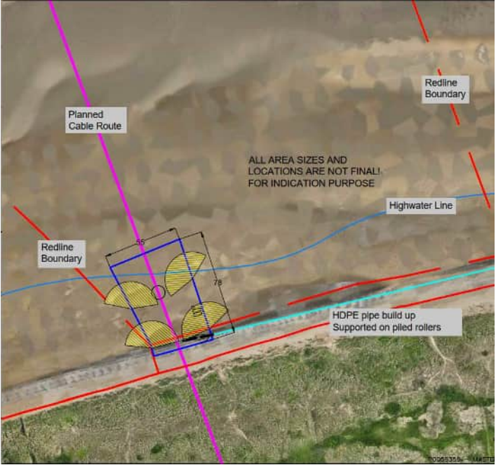
Figure 6.2: Indicative proposed lighting scheme during construction at HDD Exit Pit
