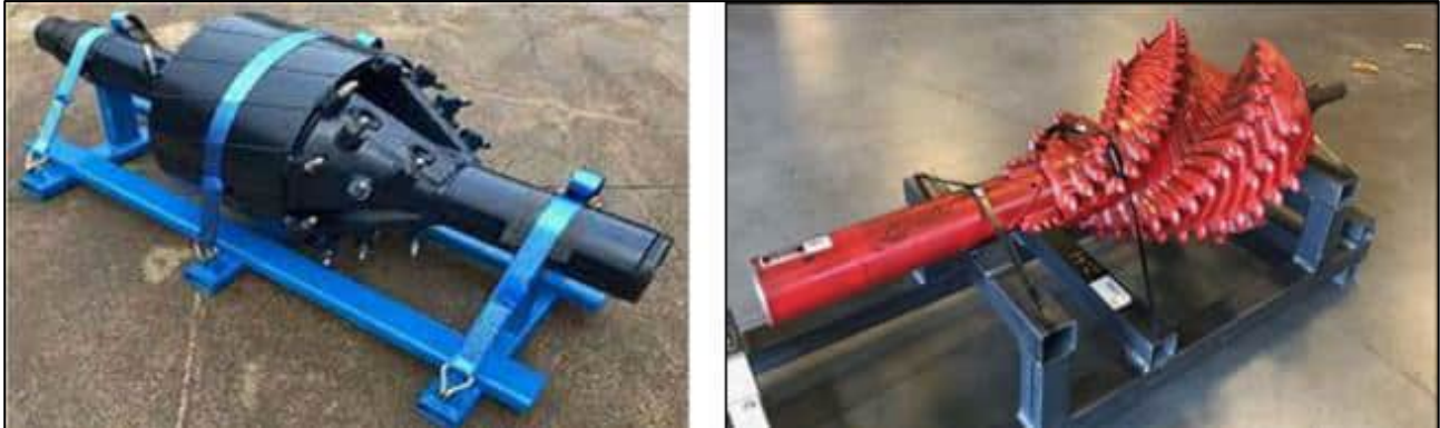
Figure 4.13: Rear reaming assembly
