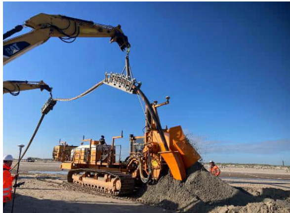
Figure 4.22: Tracked cutter trencher for onshore and intertidal burial
